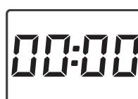
With this display, enter the time in the format HH:MM using the rotary controller, and confirm by pressing the rotary controller. Each value can be changed when it flashes.
