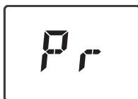
**Pr** is displayed. Press the rotary controller.
