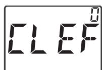
Press the key and rotary controller simultaneously for 3 s until **CLEF 0** is displayed and the symbol disappears.
