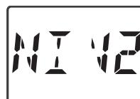
Press the and keys for 3 s until **NIV2** is displayed. Press the key for 3 s until the first parameter is displayed. Press the rotary controller to move onto the next parameter and, at the end, to return to manual operation.
