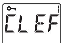
Press the key and rotary controller simultaneously for 3 s until **CLEF 1** and the symbol are displayed. The device is now protected against unauthorised access to the settings and only the on/off key and the blower can be activated.
